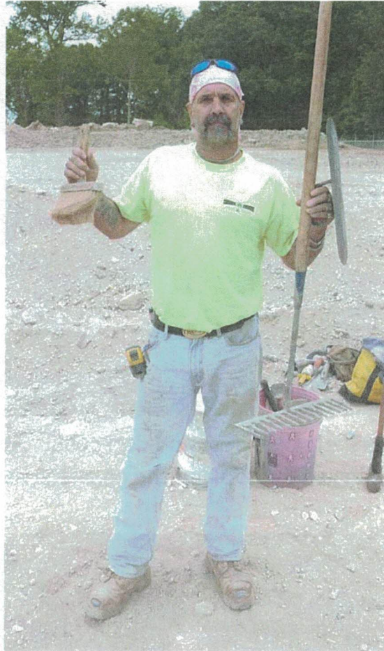
Some of the tools you should not use – a brush for blessing concrete, a rake for moving concrete, and a steel trowel.
