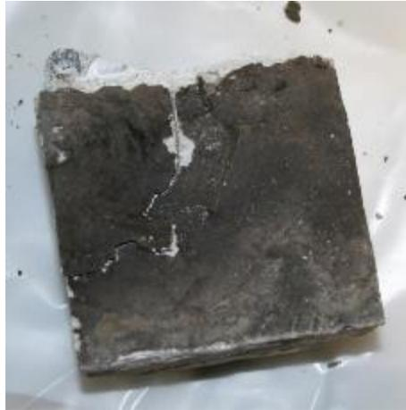
**Figure 49.** The black material within the crack seems to be a sealer such as linseed oil (Core C1\_8407\_C)
