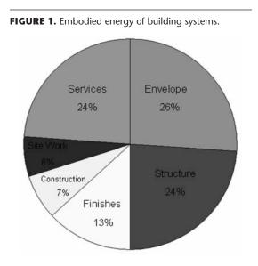
(8.7 million Btu/ton). When we compare the embodied energy of various building systems, we find that the embodied energy of concrete in its basic form is much less than that of steel but greater than timber. However, when we compare the quantity of steel and quantity of concrete required to construct a structurally similar building, the embodied energy differential between the two materials disappears (Sustainable Design Resource Guide, 2008).
