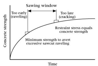
If using an early entry saw, cutting may be possible within a few hours of placement. Research has shown that the timing of the saw cut is more important than the actual depth of the cut. Although shallower depth may be utilized, industry standards still recommend cutting to a depth of 1/4 the thickness of the slab.
