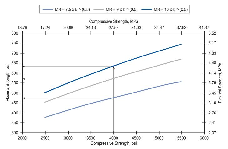
Figure 1. Plot showing the range in correlation constants for compressive to flexural strength conversion. Exact correlation constant will be mix-specific.
