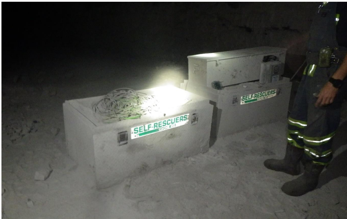
Figure 13. SCSR cache and tetherline storage.
