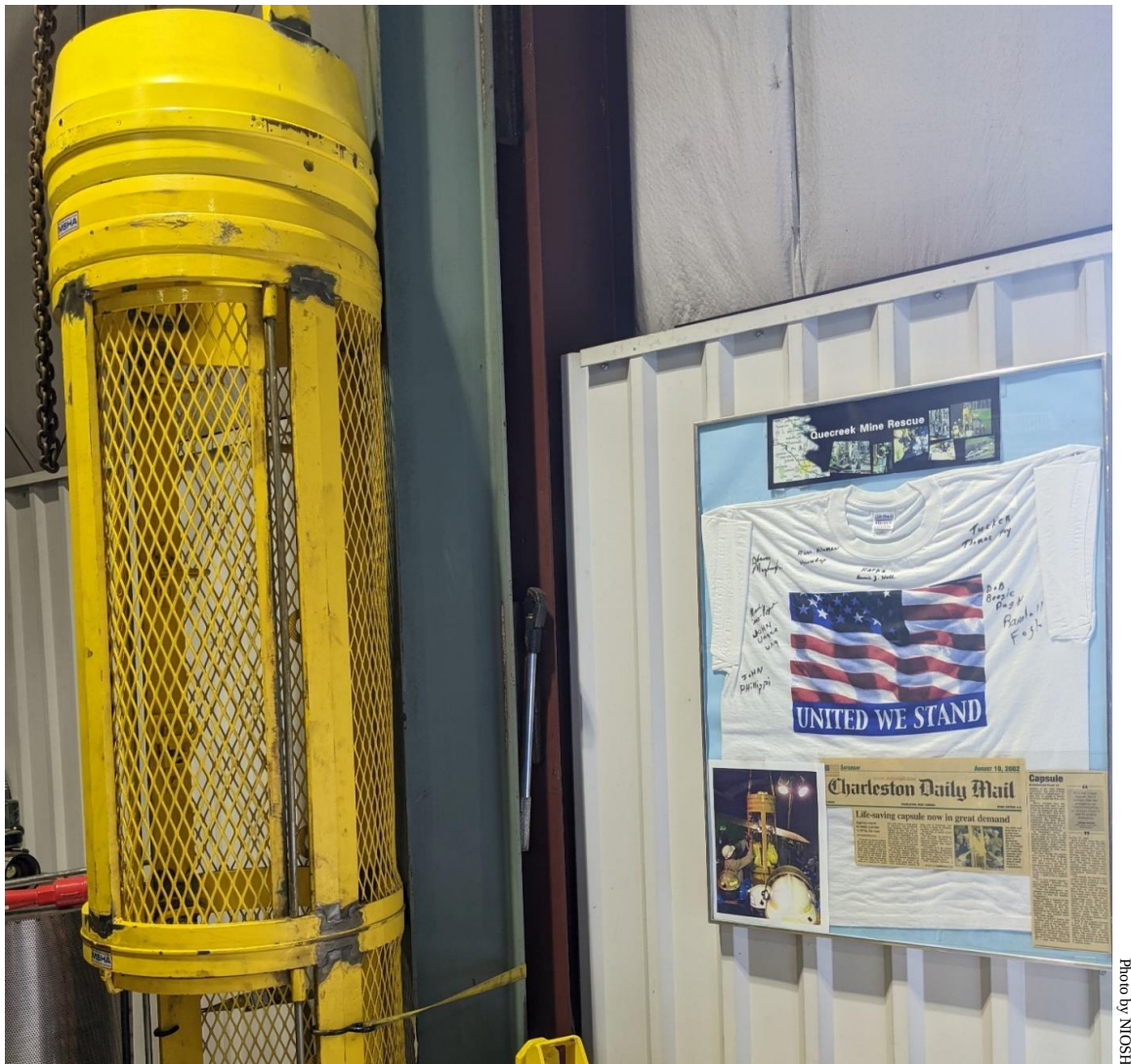
Figure 8. A rescue capsule similar to the one used to rescue nine miners at Quecreek in 2002 and a display commemorating the rescue at the MSHA Academy in Beckley, WV.
